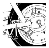
**7** Tighten the brake housing anchor securely.
